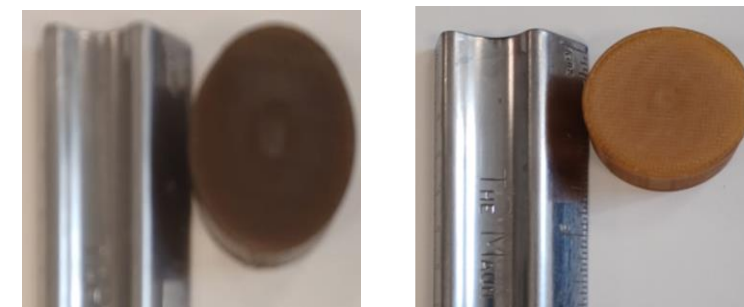
Figure 4 – Erosion samples after impingement
