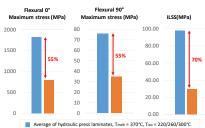
Average of hydraulic press laminates, Tmelt = 370°C, Tiso = 220/260/30 ATP laminate, Tnip = 360°C, Ttool = 25°C, Vroller = 4m/min, Proller = 2 bar
