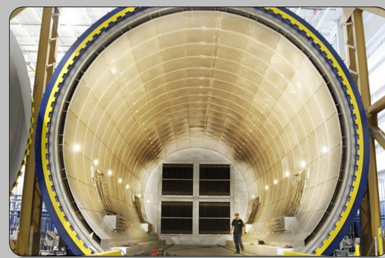
Figure 1. A giant autoclave for baking CFRPs (aviation-images.com)
