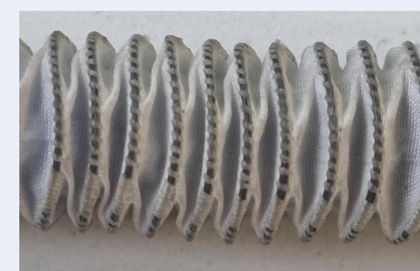
Fig 5 Anaconda Leg in Compression
