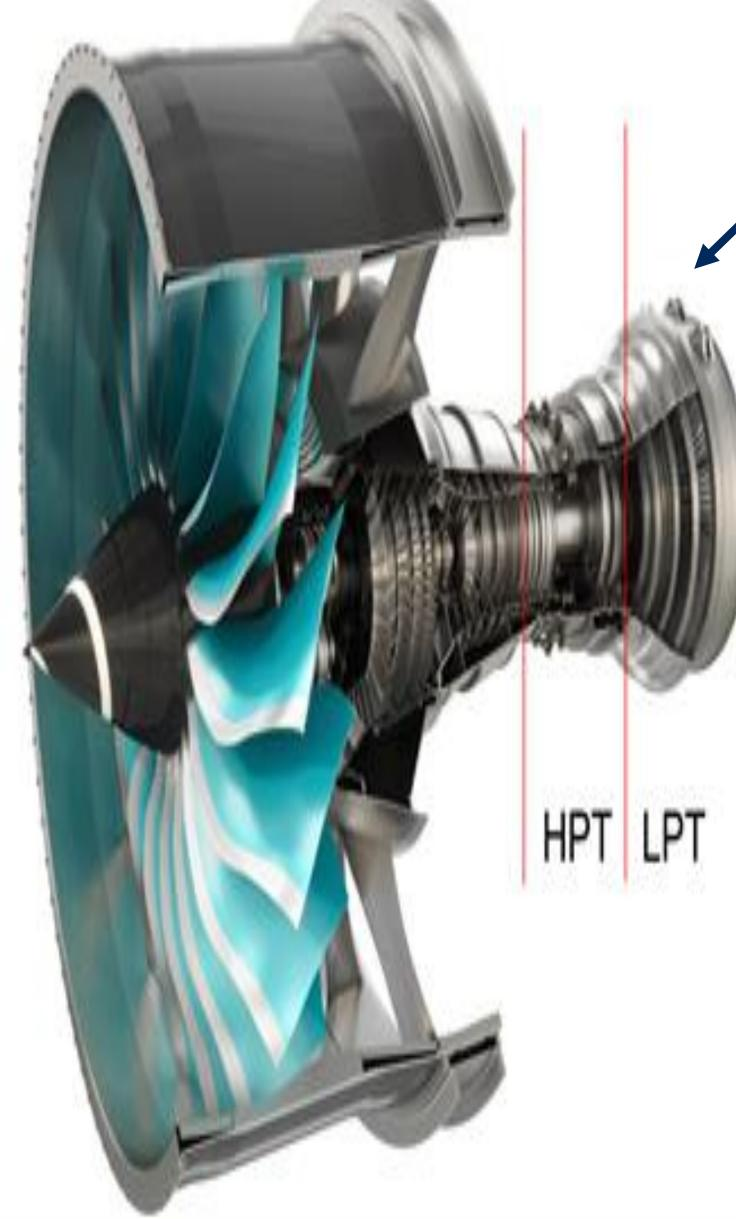
**Rolls Royce, Pratt &** Whitney and GE all apply different TiAl alloys to their turbine low-pressure (LPT) blades<sup>1,2</sup>
