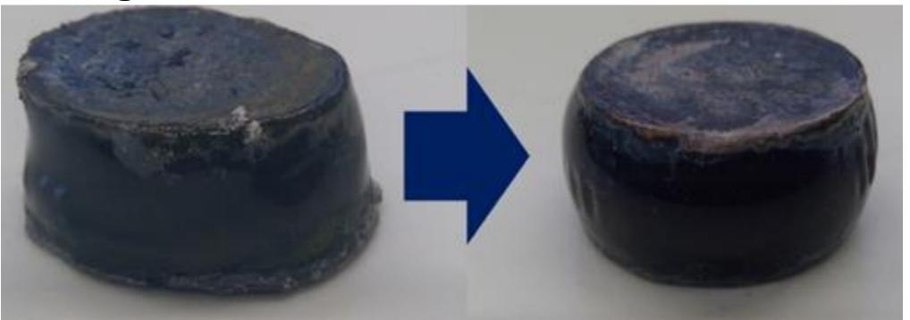
The aim of our work in an image, improving forgeability of these cast alloys
